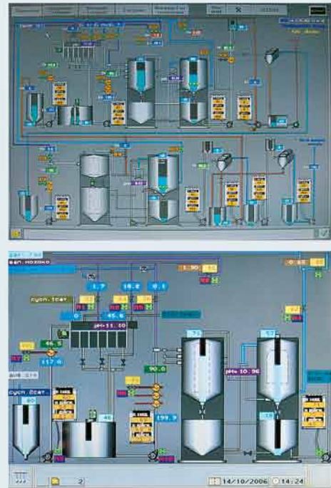
Purification Station Control System Mnemonic Diagram
