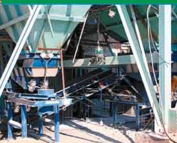
General View of the System for Feedstock Preparation and Loading to Skip
