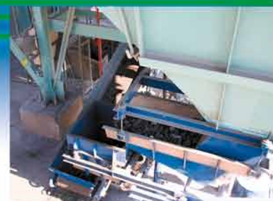
Fuel Vibratory Dosing Feeder
