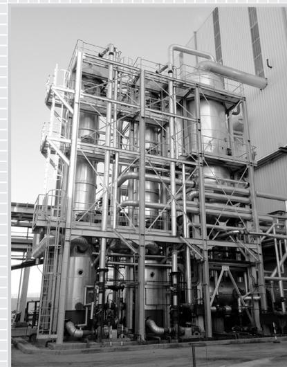
Design and installation of evaporation station for La Belle Sugar Refinery in Algeria
