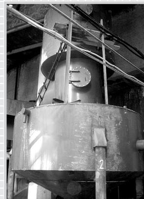
In terms of design, the burner consists of a refractory-lined cyclone muffler fitted with a air-supply unit and a spray nozzle. An air distribution chamber is divided into compartments and composed of a conical swirler with cone parts eccentrically positioned along the axis for air injection, which ensures efficient ignition of coal-water fuel and its complete burnout in the muffler chamber.
